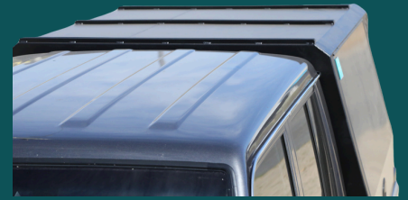
Unistrut Rails on Roof
